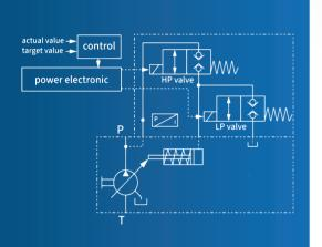
Today, different types of mechanical pump controllers are used for different applications. Through the development of a patented digital pump controller HPC, we are engaging the future. HPC enables the option to control all types of piston pumps with only one controller. The passive component "hydraulic pump" becomes an active system device that communicates with the machine. The HPC is designed as a pump smartifier. Based on this technology a more efficient and flexible system is possible.
